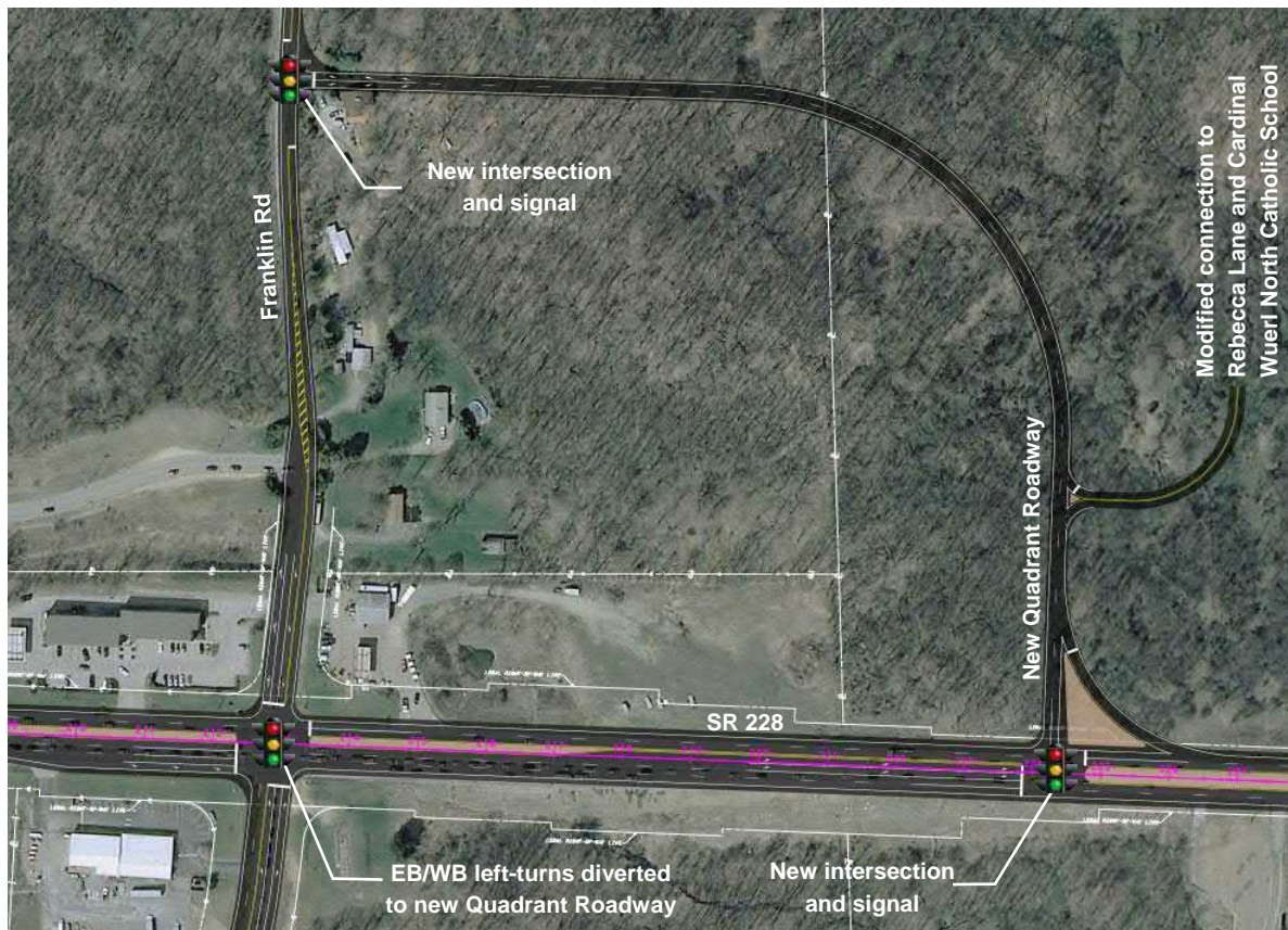
Exhibit 26: SR 228 at Franklin Road – Quadrant Roadway Concept
